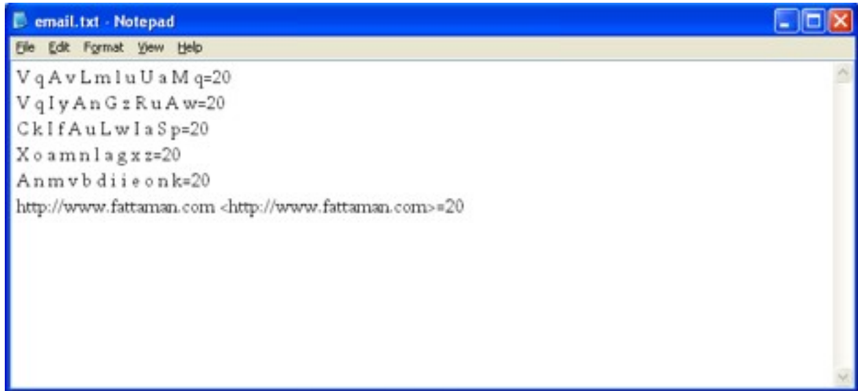
Figure 6: This email scored 17.2 by SpamAssassin. Although the text of the body of this email is confusing to users (In fact, spammers can use a Java script to remove those small letters among capital letters before receivers read this kind of emails), it is tagged as spam by SpamAssassin. Especially, the link is in SpamAssassin's blocklists, which make it have a higher score.
