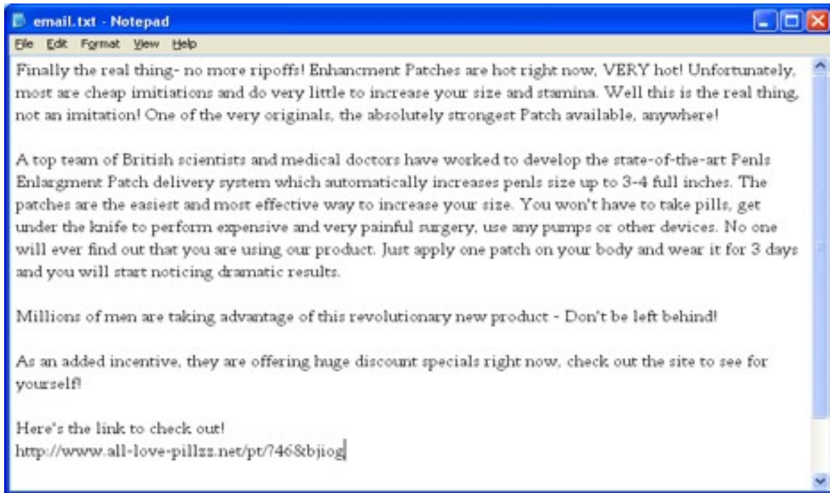
Figure 14: The original spam message before obfuscation. We can see that the spammer has changed the form of the keyword "penis" as "pen1s" and "penls" and misspelled "enlargement" as "enlargment", trying to bypass spam filter. However, after being trained, SpamAssassin can block this.
